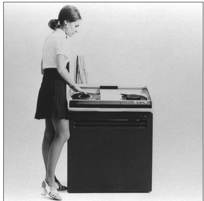
IBM 3410 magnetic tape system with horizontal tape insertion option
