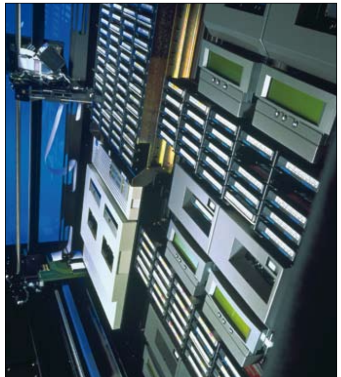
IBM 3494 housing unit D22 with 'Cradles' and TS1120 (Jaguar) drives
