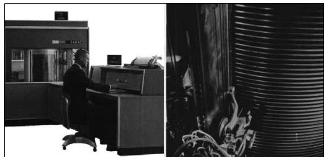
IBM 350 RAMAC plate, 51 plates in a 24 inch diameter stack. 1956: 5 MB model (5 million 'characters'), 1958: 10 MB model (10 million 'characters'), withdrawal from sales in 1960
