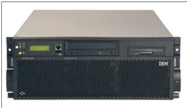
IBM NAS Gateway 500, available February 2004, pSeries-based, up to 224 TB capacity in the SAN
