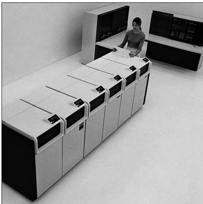
IBM 3350, capacity up to 2,536 MB, 317 MB per LW, 8 drives per 3350 line, access time 25 ms, data rate 1,198 KB / s, left rear: display unit for microfiches, right rear: control console of the system / 370 model 168
