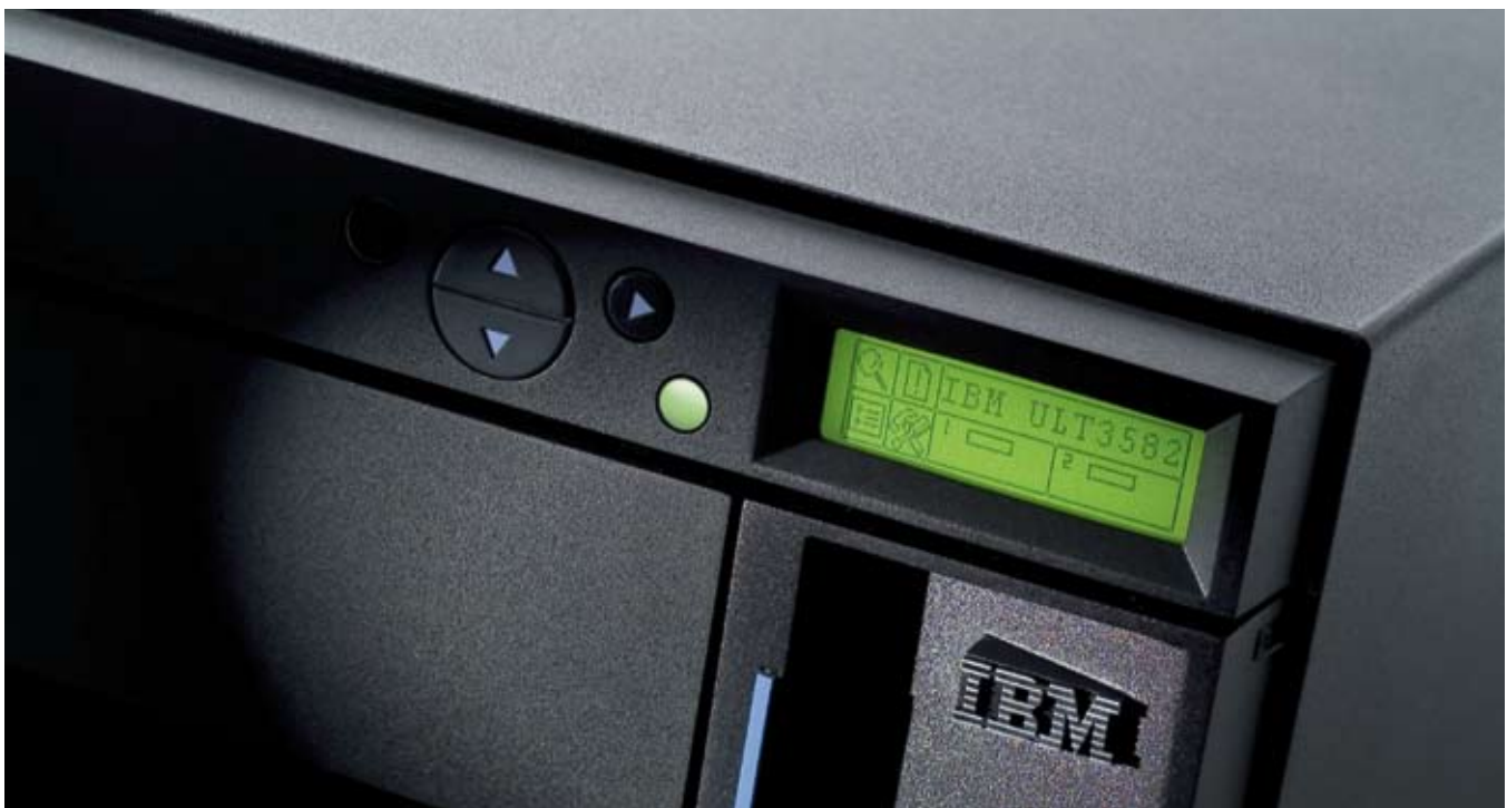
IBM 3582 Display - mini library with up to 23 LTO cartridges
