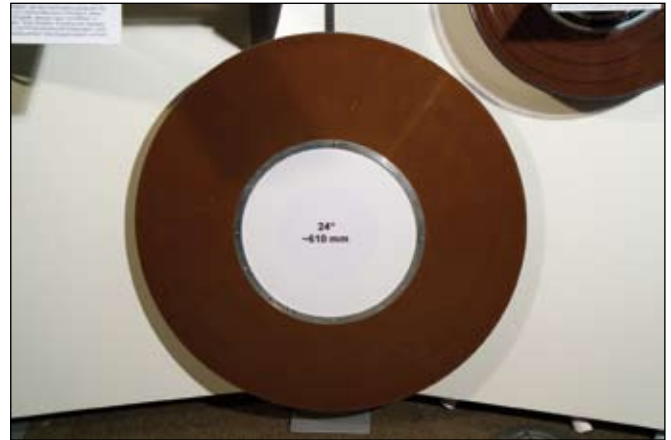
IBM RAMAC 350/355 plate with 24 inch diameter years 1956-1957
