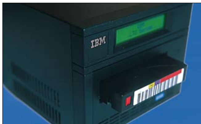
Cartridge loading on the IBM LTO1 drive
