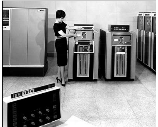
IBM 7340 Hyper Tape Drives in the center of the picture, on the left the IBM 7640 control unit, on the right the IBM 729 tape units
