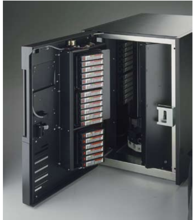
IBM 3583 Ultrium Scalable Tape Library with the door open
