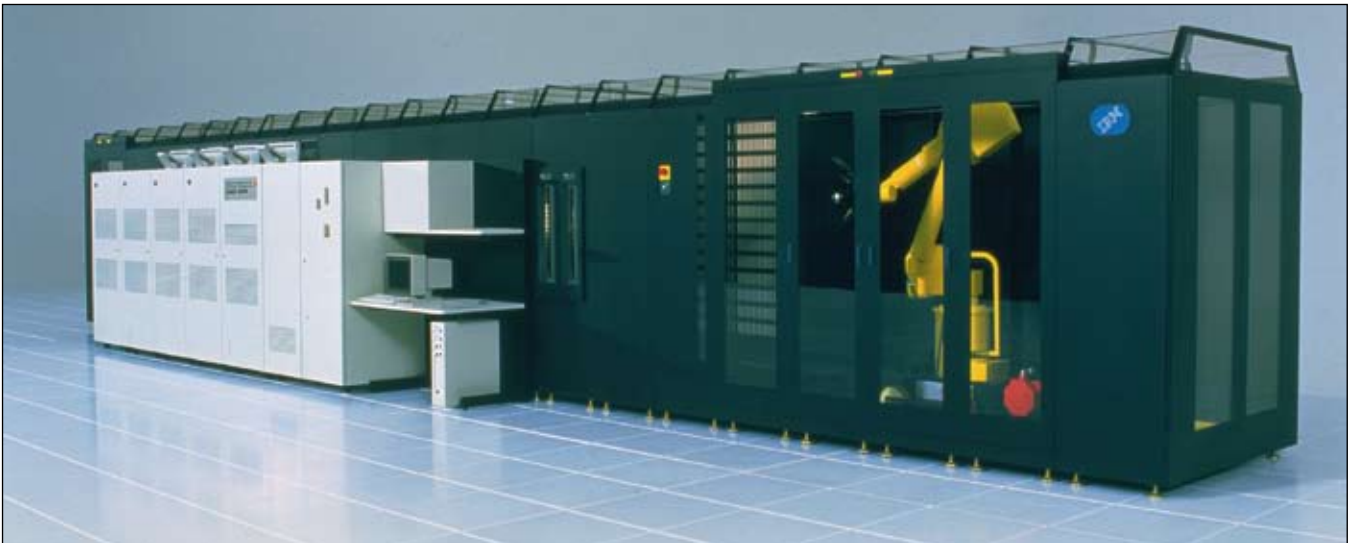
IBM 3495 tape archive with 5,660 to 18,920 cartridges (13.5 to 45.5 TB), height 2.38 meters, depth 2.46 meters, length depending on the model 13.4, 18.3, 23.2 or 28.0 meters, 4 to a maximum of 64 IBM 3490 drives
