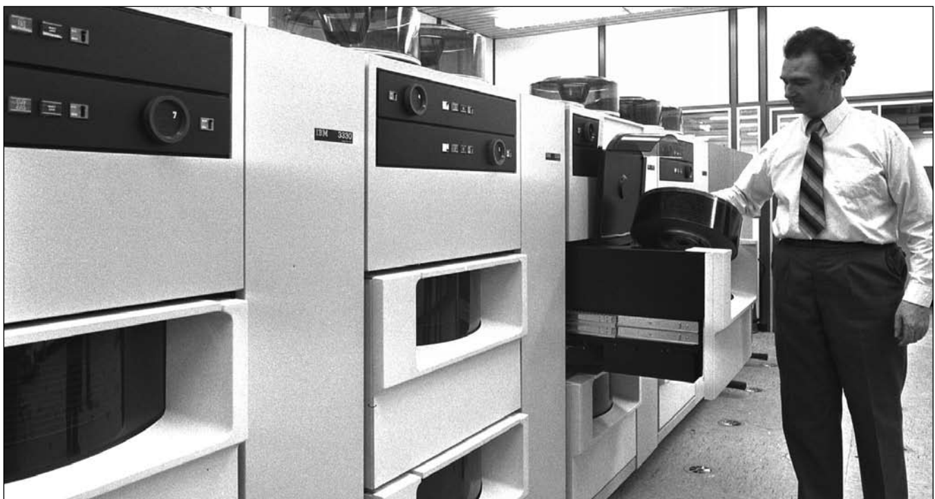
IBM 3330, capacity 800 MB, 2-8 drives, access time 30 ms, data rate 806 KB / s, announcement model 1 on June 30, 1970, model 2 on October 4, 1972, model 11 on July 17, 1973, withdrawal from sales on December 20, 1983
