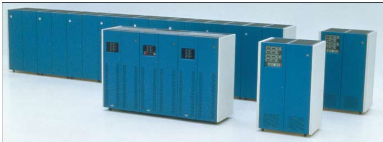
1989: IBM 3390-1 / 2, 1991: IBM 3390-3, 1994: IBM 3390-9, rear IBM 3380-K line with 60 GB capacity, front 3390-3 line with 90 GB capacity, right IBM 3390 control units
