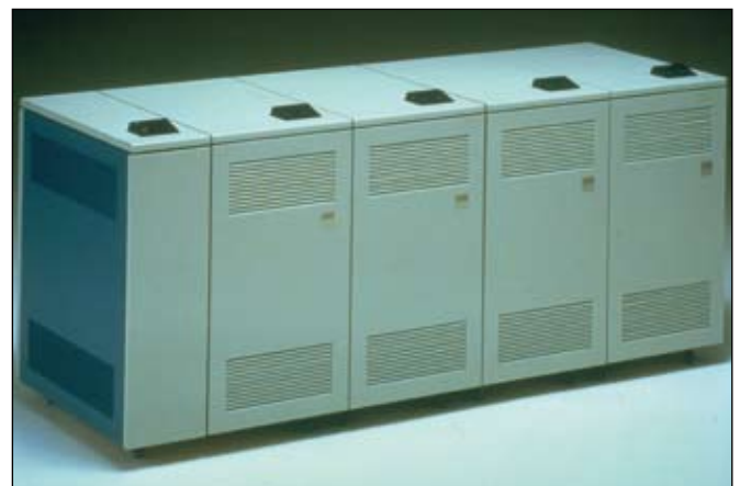
IBM 3370, 1 disk stack per unit with 2 access arms and 2 addresses, model 1: 571 MB, model 2: 730 MB, each per unit, up to 4 units with 2,285 - 2,920 MB capacity, access 20 ms, data rate 1.86 MB / s
