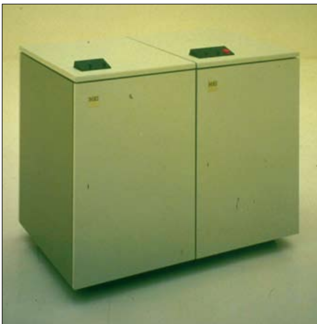
IBM 3310 Direct Access Storage, disk system for IBM 4331 computers
