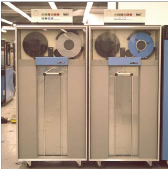
IBM 3420 magnetic tape unit, 1970 models 3, 5 and 7, 1973 models 4, 6 and 8
