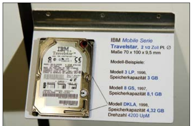
IBM Travelstar 1996-1998 as a mobile plate in laptops
