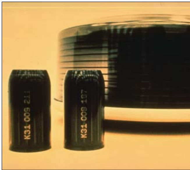
IBM 3850 tape cartridges with 19.5 meter tape length and a capacity of 50 MB each in size comparison to the 3330 plate stack with 100 MB capacity
