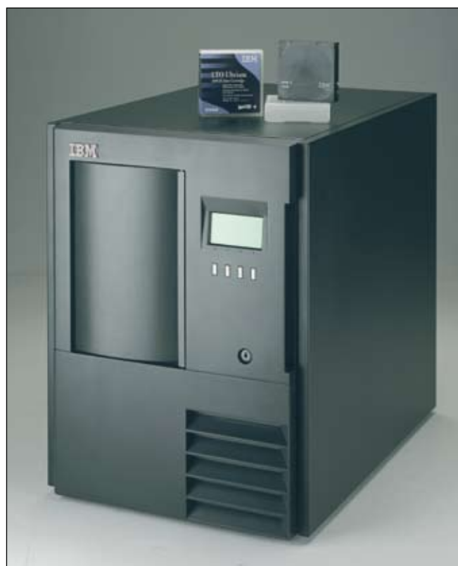
IBM 3583 models L18, L36 and L72, capacity with LTO1 cartridges up to 7.2 TB (native), ADIC sold the product as Scalar 100 under the ADIC logo
