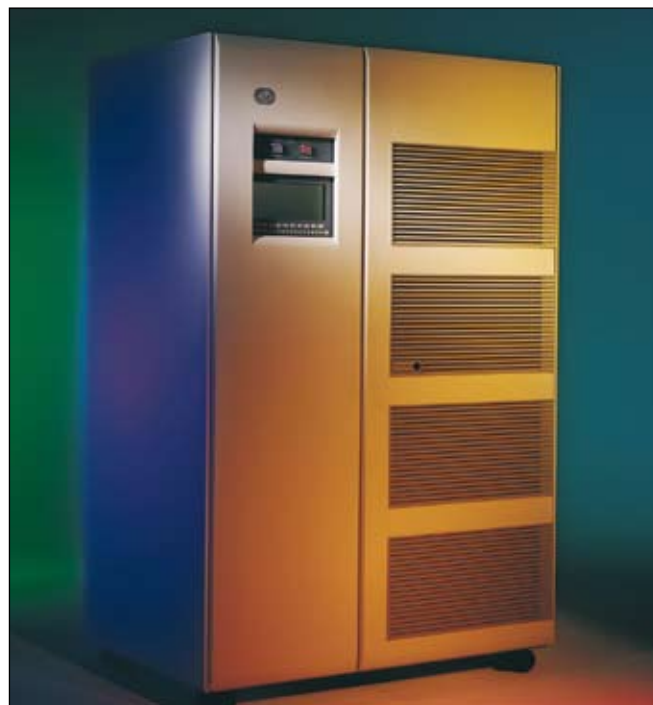
1996 - 1998 IBM RAMAC Virtual Array RVA, IBM RAMAC Virtual Array 1996, IBM RAMAC Virtual Array Turbo 1997, IBM RAMAC Virtual Array Turbo 2 1998, capacities from 840 GB to 1,680 GB arrays 13 + 2 + 1 RAID6 or 2 x (5+ 2 + 1), array capacity up to 420 GB, minimum configuration: 2 arrays, maximum configuration: 4 arrays
