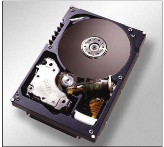
IBM Ultrastar 146 GB drive with 10,000 RPM
