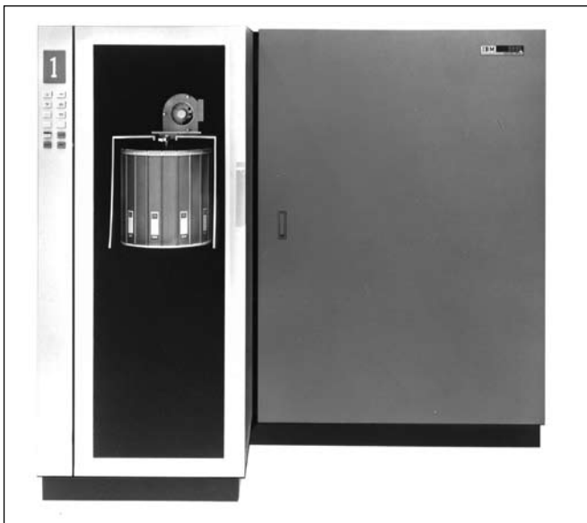
IBM 2321, total capacity of 400 MB, expansion levels of 40 or 80 MB, access times from 95 to 600 ms
