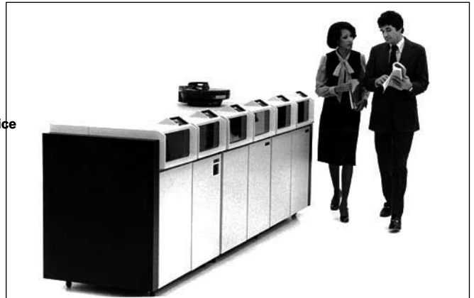
IBM 3340, maximum capacity up to 4,800 MB, Winchester removable disks model 35: 35 MB, model 70: 70 MB, up to 64 drives (models 158, 168), data rate 885 KB / second, access time 25 ms
