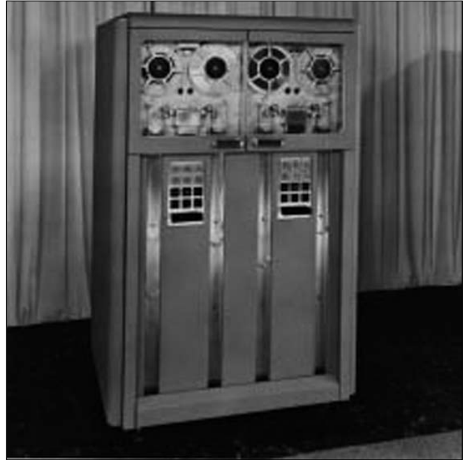
IBM model 726 magnetic tape unit, launched in 1952
