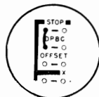
Figure X-6. Double-Punch and Blank-Column Detection Wiring
