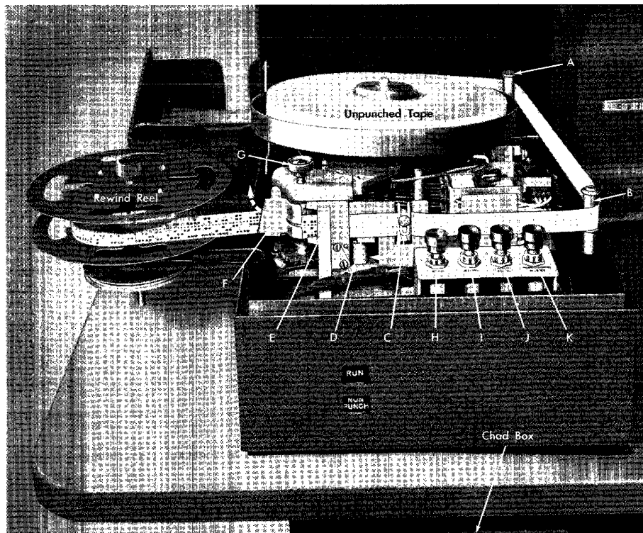
FIGURE 11. TAPE PUNCHING UNIT WITH COVER RAISED FOR TAPE THREADING
