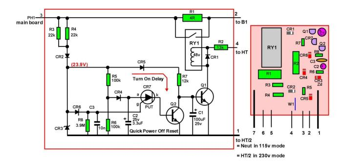
IBM - 5155 POWER SUPPLY - INR USH CURRENT LIMITER
