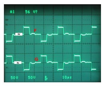
A recording at the comparator output H is shown below, the voltage only rises to about 1.4V due to the base-emitter junctions of Q1 and Q2. Notice how this circuit is switching at twice the supply's fundamental 28.5 KHz:
