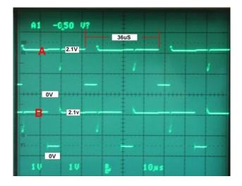
Of note the frequency of operation of this supply is close to 28.5kHz. This is slow compared to many modern computer switch-mode supplies. However, it has the advantage that there are less switching events per unit time, so the efficiency is a little higher and probably the high frequency harmonics do not extend as high up into the radio frequency spectrum.
