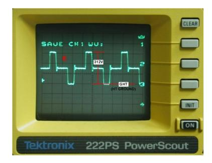
Notice how this output waveform (from Transistors Q1 and Q2) has a 156V DC offset. Before this waveform can drive the main transformer T1, this offset must be eliminated. This is the job of capacitors C2 and C4 which will be seen later on the circuit which includes T1 and the output filter components.
